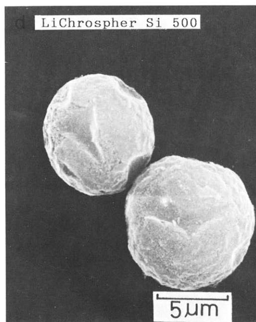
Fig. 1. TEM photographs of (a) porous glass and (b and c) LiChrospher Si 500 and (d) SEM photograph of LiChrospher Si 500.
